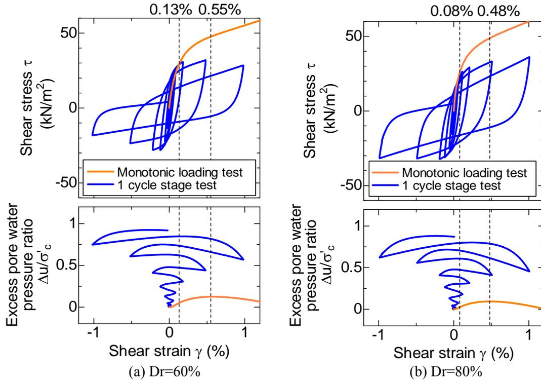
Figure 3. Relationships between Shear stress and shear strain, and excess pore water pressure ratio and shear strain obtained from monotonic loading tests and 1 cycle stage tests.
