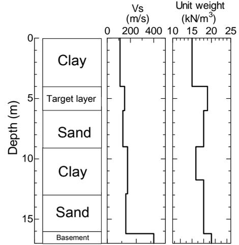
Figure 5. Model ground for hybrid and usual ground response analyses.
