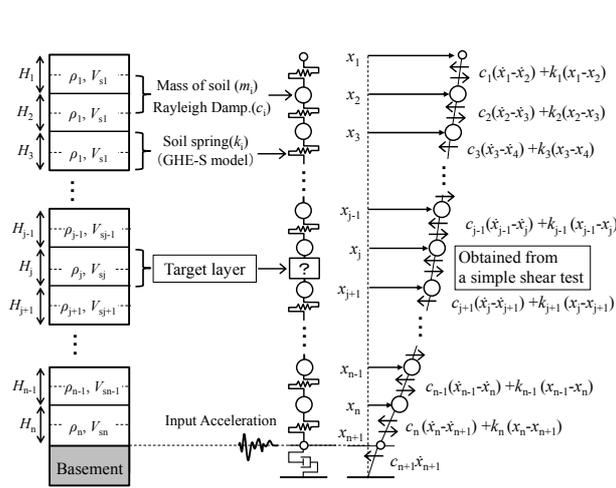
Figure 4. A conceptual figure of a hybrid ground response analysis (HGRA).
