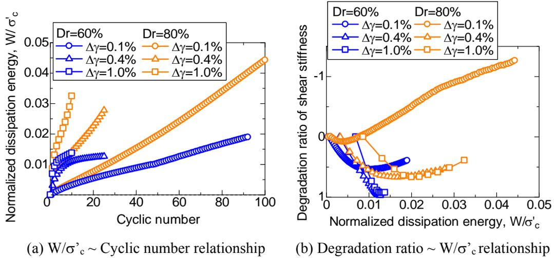
Figure 2. Results obtained from constant strain cyclic loading tests
