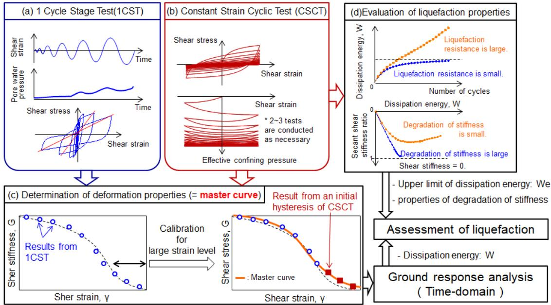
Figure 1. Concept of the proposed testing method.
