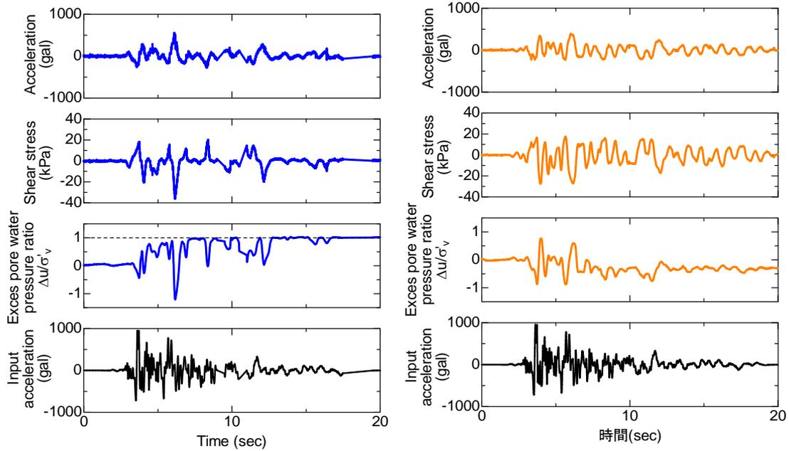
Figure 8. Time histories of seismic response obtained from the HGRAs
