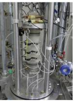
Hollow cylindrical torsional shear test
