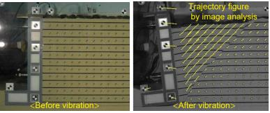
Case① Shaking tablet test of abutment model
