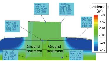
Case① Study of liquefaction counter measures for L2 earthquake (SENPS)
